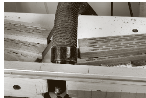
Keep track of where you are by using two stacks of material as you work through the progression of cuts.
