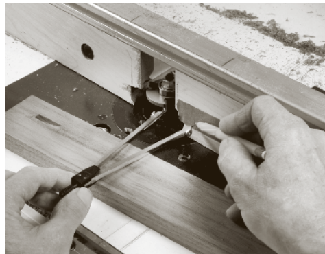
The first mark is made from the point in the cutting arc that intersects with the plane of the fence.
