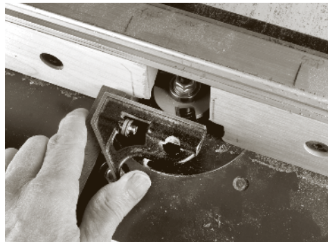
The easy way to set the depth of cut is with a combination square. Set the blade at the desired increment and when the bit kisses the blade, it's right.
