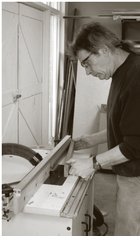
Begin each cut by placing the end of the board against one of the marks on the fence.
