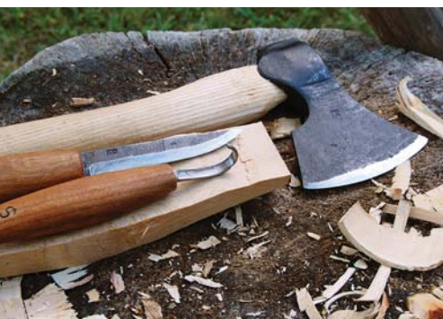
Tool kit. It takes only a few tools to shape your own spoons; I use a hatchet and two – sometimes three – knives.
