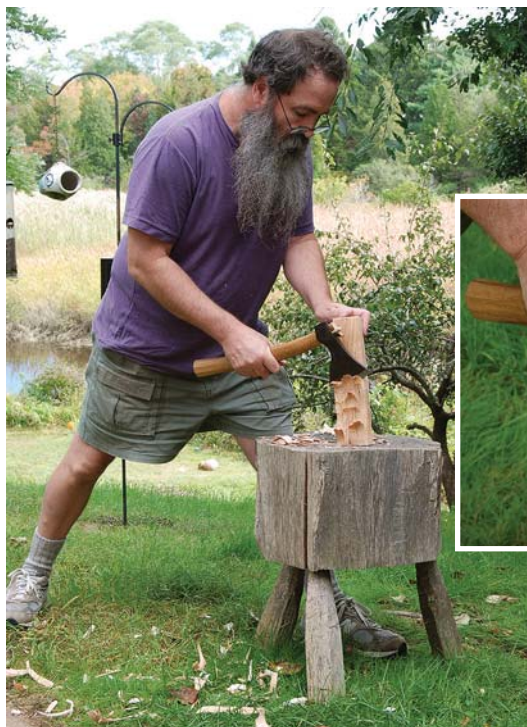
Safety stance. To keep your hands out of harm's way, work at the proper height with the cut angled away from your body and into the chopping block.
