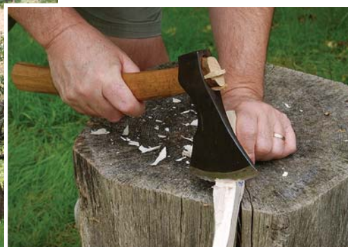
Built-in stop. A notch in your block gives you more control over detail chopping work.
