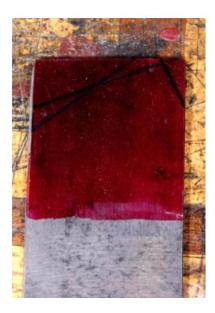
Set the iron forward so it protrudes to its full width. Use a long thin awl to scribe the plane profile onto the iron, and keep the awl as flat as possible on the bed. Make one scribe mark for each face of the profile. Remove the iron from the plane, and clean up the scribe marks.
