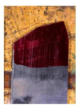
To check my progress, I hold the iron firmly to the bed with my thumb with the plane upside down and the toe facing to me. I then advance the iron to just peak over the sole (keeping the iron centered in the bed). The face of the iron is red from the layout fluid, but the newly ground, blunt edge is shiny. Take care to only judge the iron profile from the red face. The fillet edge can be ground to close to its final dimension, but leave it fat (at least 1/16° shy of the final edge).
