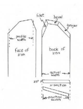
The second bevel should have the same width as the first bevel. Tweak this bevel until the arris is sharp and hits the intersection of the two bevels. Grind the fillet edge to a steep bevel, but hold this well short of the final dimension.
