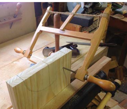
Cut. I used a frame saw to cut the half-rounds; note the relief cut in the center. You could also use a coping saw or, of course, a band saw to make these cuts.
