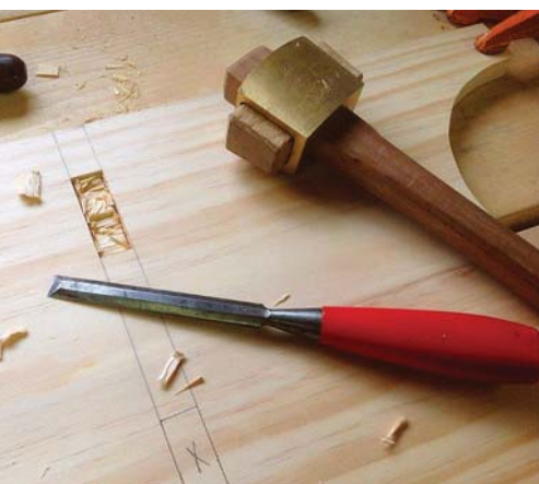
Whack 'em. With just four mortises to cut – and in soft pine, to boot – I used a chisel.
