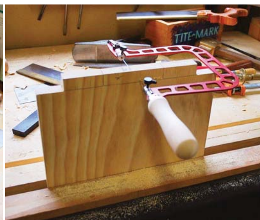
Cut then cope. A dovetail saw makes quick work of the cheek cuts, and a coping saw removes most of the shoulder waste. The rest is cleaned up with a chisel.
