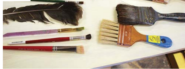
Tools. Feathers, sponges, brushes and even paper and plastic bags can be used for faux graining.
