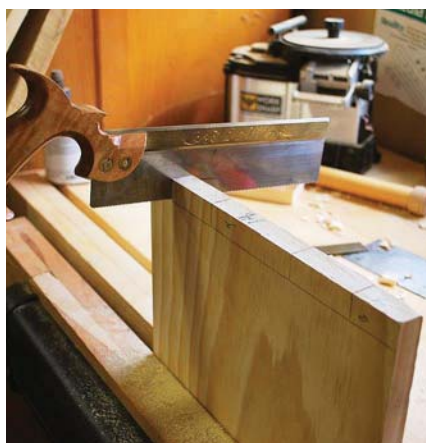
Cut then cope. A dovetail saw makes quick work of the cheek cuts, and a coping saw removes most of the shoulder waste. The rest is cleaned up with a chisel.
