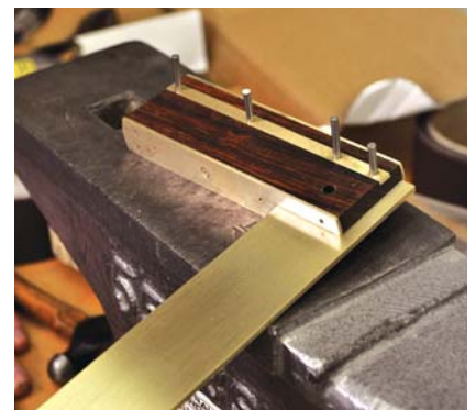
18 Only slightly proud. The rivets should be only .0625" longer than the handle thickness. Insert rivets into the holes as shown.
