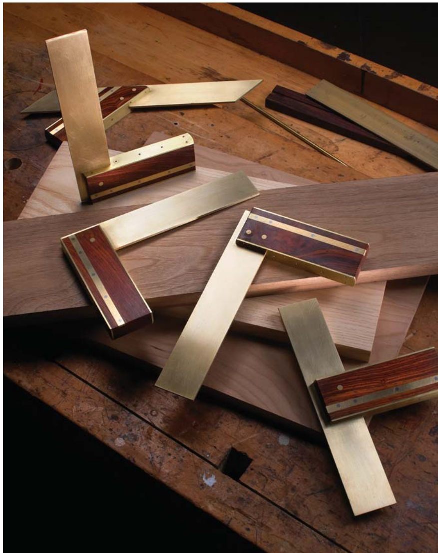
Student work. These beautiful try squares were made by John Economaki's tool-making class at the Marc Adams School of Woodworking.
