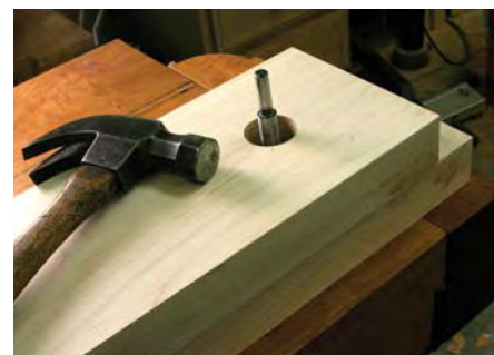
Tap then tap. Place the front jaw on the rear jaw. Drop your Forstner in the hole. Tap it with a hammer. Then drill the hole in the rear jaw and tap that.
