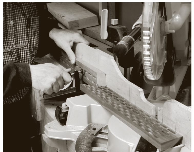
A stop block on the miter saw will keep your parts at a consistent length.
