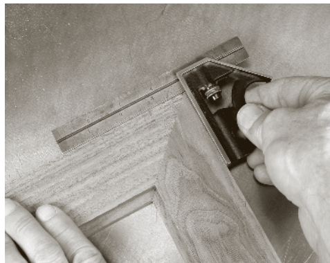
Check an assembled corner to be certain it is square. Place the material on a flat surface and use a reliable square.
