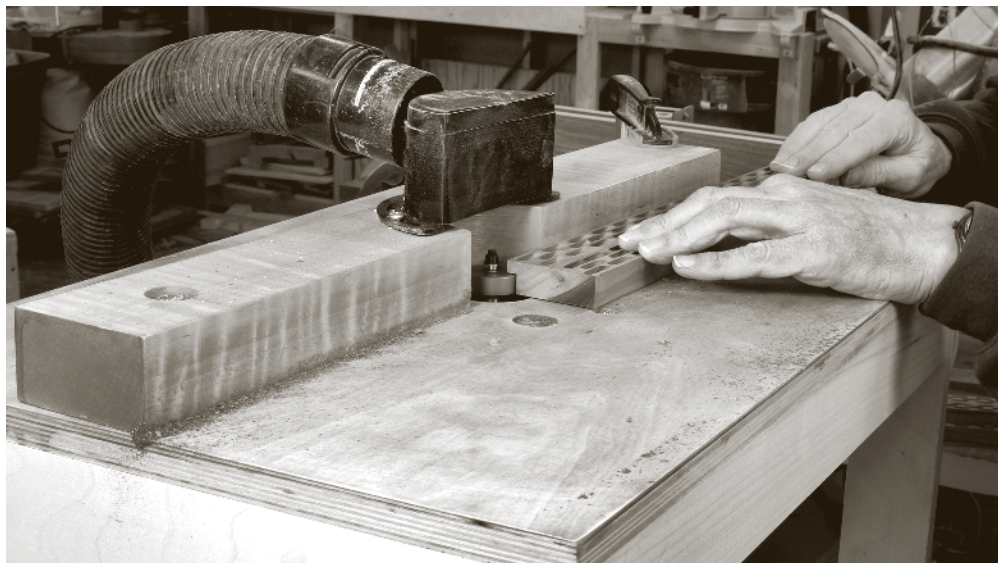
The rabbet in the back of the frame material doesn't need to be wide, but it must be deep enough to fit the glass, mat and foam board.
