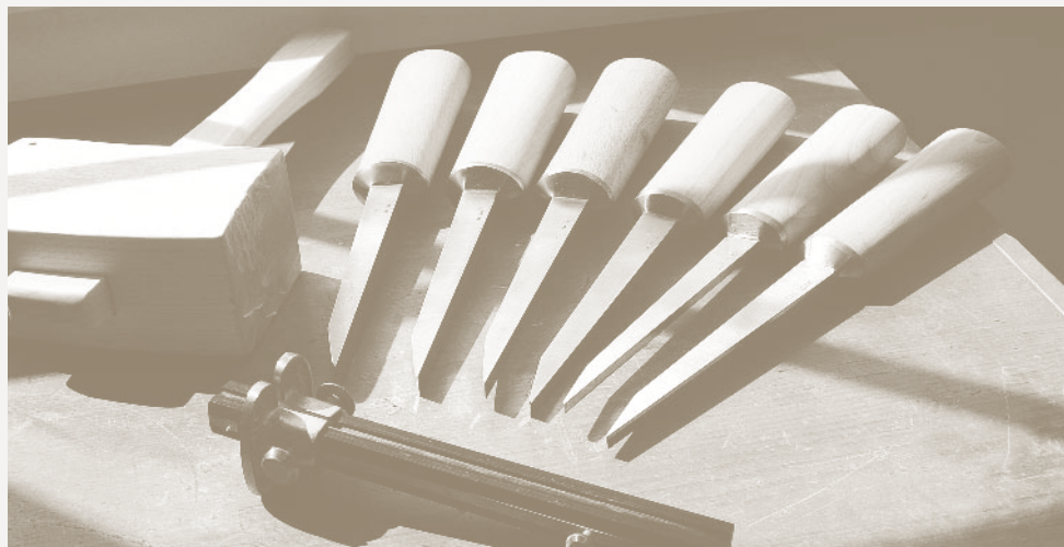
The Ray Iles mortising chisels revive a pattern of tool that has been lost for decades. They work remarkably well, outcutting other chisels in our shop.
