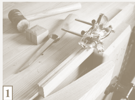
1 I cut the grooves for this drawer with a little plow plane. Its 1/4" iron is exactly the same width as my mortising chisel. My chisel also matches the groove made by our shop’s 1/4" straight bit.
