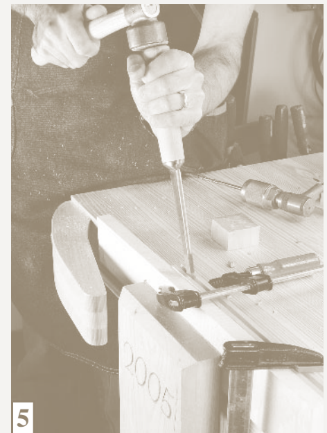
5 Again, note the stance and the two clamps involved in mortising. This clamping setup keeps the work from shifting to the side or pulling up off the bench.
