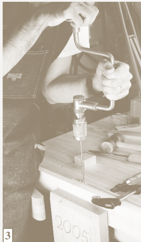
3 Note the stance here. I’m watching the bit in the most important axis. If I tip left or right, my mortise chisel will follow the hole.
