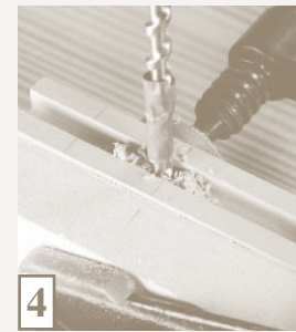
4 Generally, I mark only the auger bit with tape. The hole limits the depth of cut made with my chisel. Attempts to mark the depth of cut on the chisel are always a struggle.
