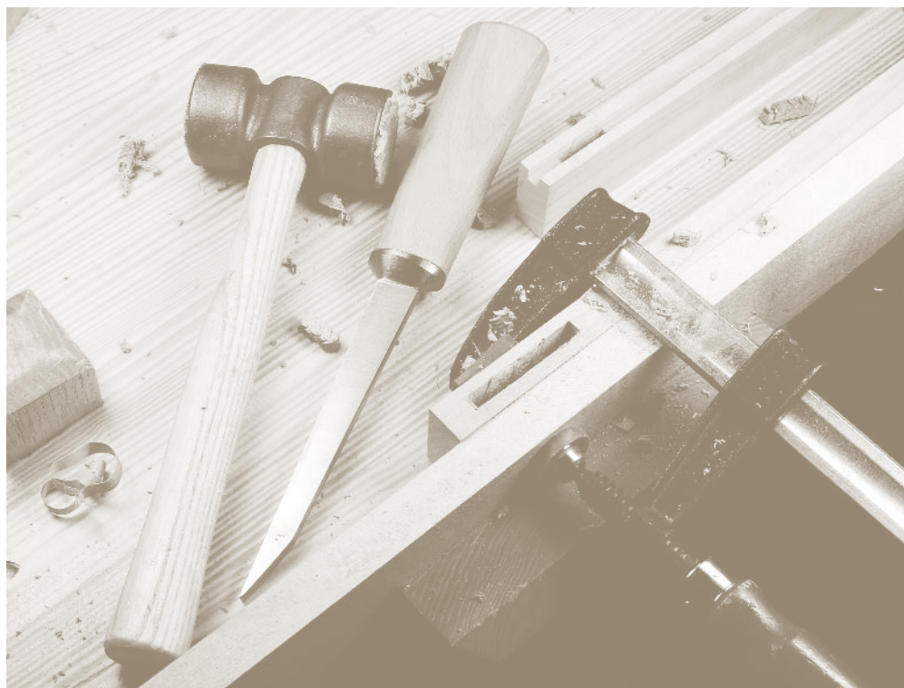
The right mortising chisel and the right technique are key to your success in cutting this joint by hand. Using a bevel-edge chisel for this technique is slow and can even snap the chisel.
