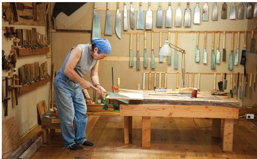
Low bench. The hipboards are cut to size by hand.
