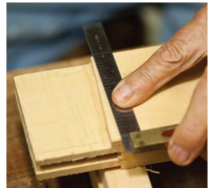
Not square. The shoulder of the dividing rail is angled to match the bead below with the bevel above.
