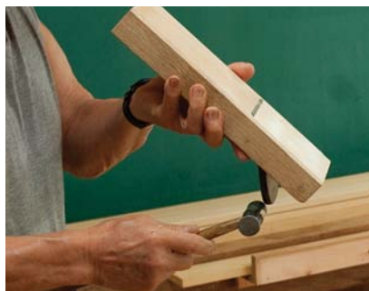
Practiced adjustment. The iron of the finishing plane is adjusted with light taps of a hammer.
