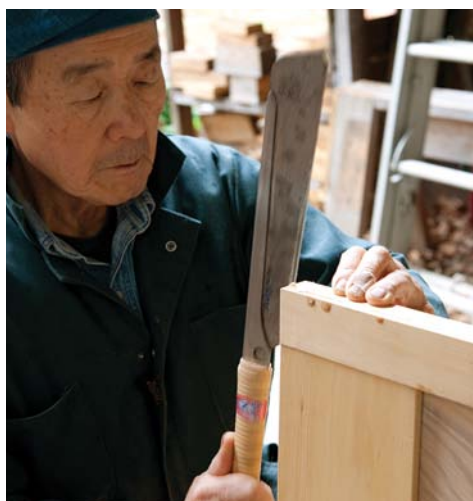
Finishing touches. A slot is cut in the bottom of the stile, allowing it to clear the rail.
