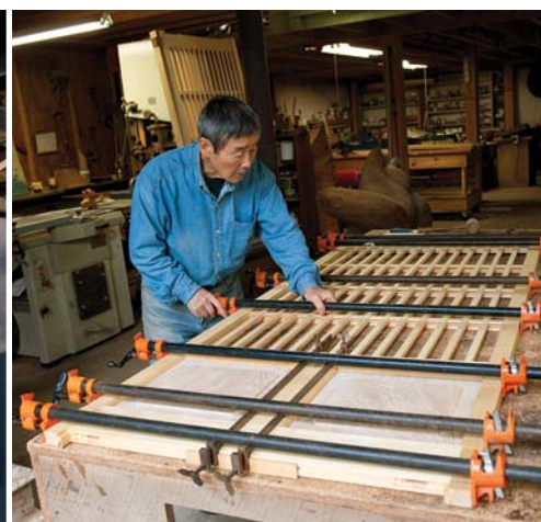
No turning back. Glue is applied and the panel is clamped together.
