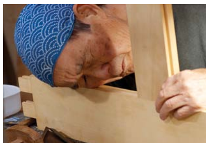
Looks right. The fit of the joint between the dividing rail and the stile is checked.
