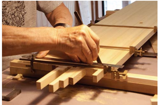
All at once. The lattice pieces are clamped together and marked for length.
