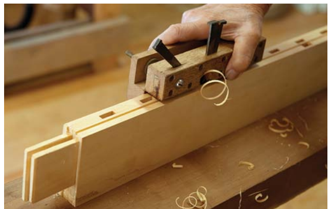
Groove for glass. The shakuri kanna (plow plane) is used to form a narrow groove for the glass panels.
