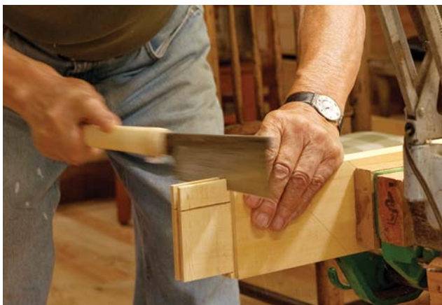
Cutting flush. The vertical shoulders of the tenon are sawn.
