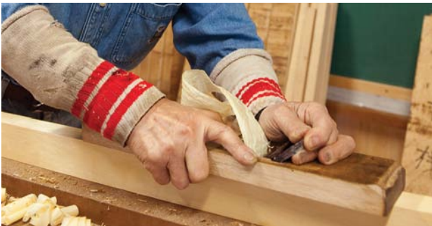
Smooth inside. The roku-dai kanna is used to smooth the inside faces of the stiles.
