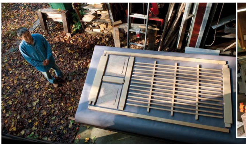
Becoming ready. All the parts for one panel are arranged before assembly.
