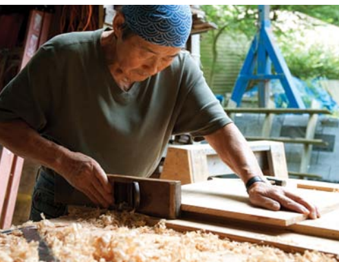
Square end. One of the raised-panel hipboards is planed square on the end.
