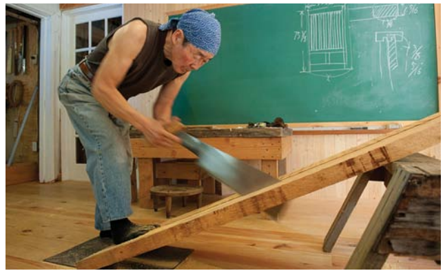
Ripping stiles. A gagari saw is used to rip the stiles from the Alaskan cedar plank.
