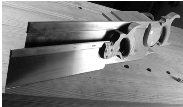
These two saws are so different in size that it’s hard to believe that they both are called tenon saws. The big saw is a much older (and almost extinct) form.
