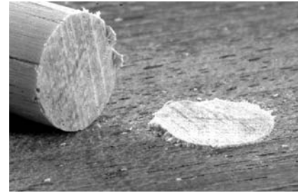
This cut started on the right. Rolling the wrist caused the blade to ride upward as the cut progressed, which resulted in a higher left side. Additional work is needed to flush the peg. Holding the wrist level results in a smooth cut.
