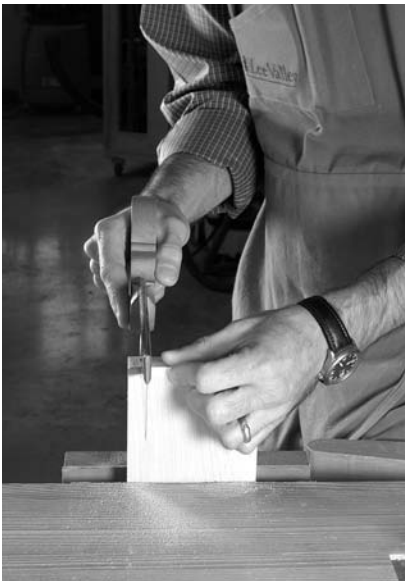
One of the most common mistakes beginning sawyers will make is they will keep their elbow tucked against their torso when sawing.
