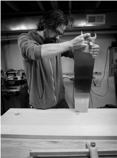
Rip then crosscut. If you rip the moulding piece first before crosscutting the front from the back, you will get a nice long piece of straight-grained stock.
