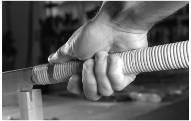
On Japanese saws the advice is mixed. Some people saw with their index finger out. Others extend the thumb.
