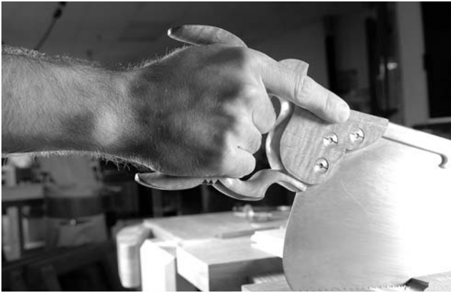
On a Western saw, it's always best to extend your index finger out along the tote. Saws are designed for a three-fingered grip.
