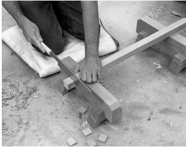
For crosscutting in joinery , the Japanese will use a dozuki (which means “shoulder of a tenon”). There are various ways to grip the saw.
