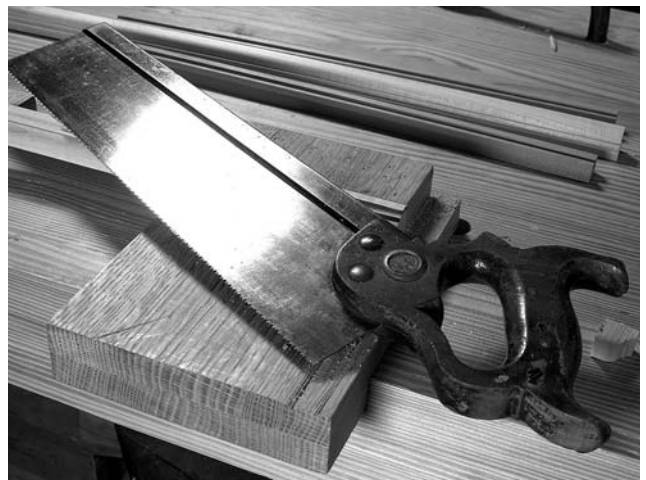
A classic vintage carcass saw from Wheeler, Madden & Clemson. This saw is 14" long and has 12 ppi. The carcass saw is used for almost all joinery crosscuts when building furniture.
