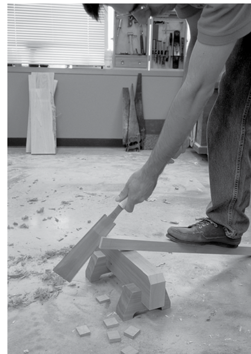
Instead of benches, Japanese craftsmen use low trestles. Sawing a tenon with a Japanese saw this way is efficient and requires sawing at a less awkward angle than at a high Western bench. However, you need to be in good shape to work this way.
