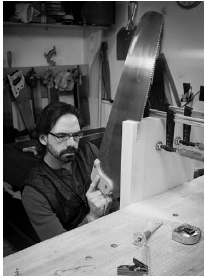
Twice as accurate. Ripping the long notches in the ends is easier if you sandwich the two pieces together. Your cut is more likely to remain square.
