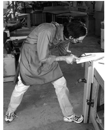
This is what a good sawing stance looks like. All the parts of my body are lined up so my sawing arm swings freely. The rest of my body is positioned in such a way that it encourages me to saw straight. Note how my toe touches the bench.
