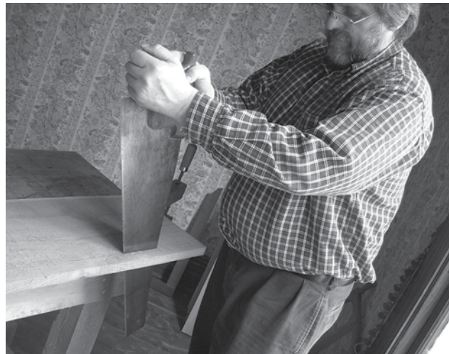
The Western handsaw, shown here being used by Don McConnell with an overhand rip grip, cuts on the push stroke.
