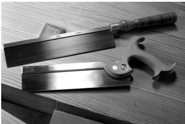
The saw on the bottom is a typical pistol-grip dovetail saw from sawmaker Mike Wenzloff of Wenzloff & Sons. Also shown (at top) is a straight-handled dovetail saw known as a gent's saw, so named (we're told) because it was used by gentlemen hobbyist woodworkers in the 19th century.
