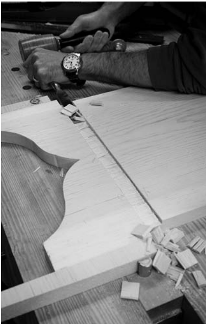
The hungry chisel. A chisel takes a bigger bite than a router plane, so do as much work as possible with the chisel.
