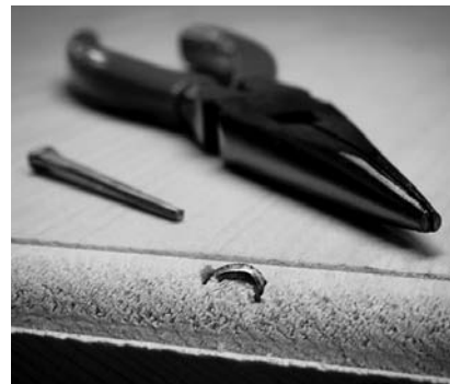
Bent over. Clenching the nails back into the moulding hooks the battens to the underside of the lid.
