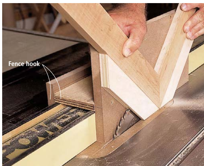
Frame splining jig
