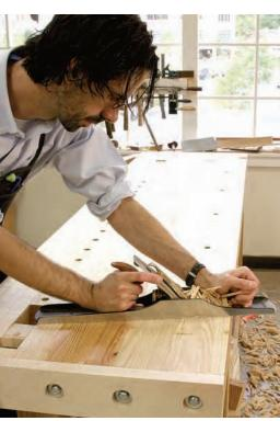
Across and down. Every stroke across the top should overlap the stroke before. The shavings will give up easily (though I am told that the iron will dull more quickly). Work from one end of the top to the other. Then back down. Repeat until the plane's cutter can touch the hollow in the middle.
