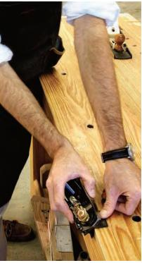
Stop spelching. Before I get down to business, I'll cut a small chamfer ( $^{1}/_{16}$ " to  $^{1}/_{8}$ ") on the long edges of the top. This will prevent the grain from blowing out (the British call this spelching) when I plane cross-grain.
