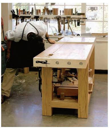
Cup or bow? Now that I know the geography of the top, I'll drag one stick all along the top and watch the gap under the winding stick. This quick check confirms my suspicions about where the high spots are (and they are usually along the long edges of the top).
