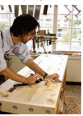
Diagonal makes a difference. Work across the top diagonally now, overlapping your strokes as before. Take care at the starting corner and stopping corner - your plane's sole won't have much support. You can proceed with speed during the middle strokes.
