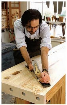
And the other way. Switch directions and work diagonally the other way across the top. Repeat these two types of passes until you can make shavings at every point in a pass.
