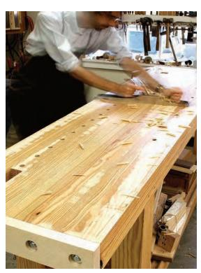
*In my cups.* In general, my tops become cupped in use. So I remove the two high hills by working directly across the grain. In this instance the cup is slight, so I started with a jointer plane. If the cup is severe, start with a jack plane so you can take a thicker shaving.
