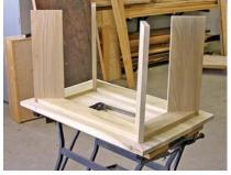
Double-check. After cutting, put the parts in place and mark the locations for the screws.
