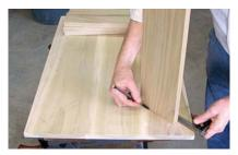
On your mark. Lay out all the pieces on the underside of the top. You won't have to measure, and all the pieces will be the exact size
