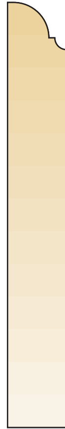
Full-scale base moulding
