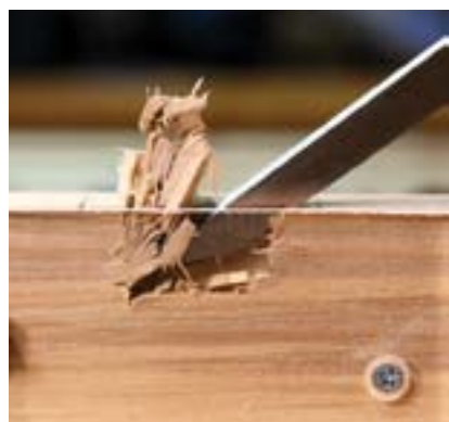
Leverage. The intersection of the bevel and the back is an effective fulcrum for levering out the waste. The sharp, square end scrapes the edges clean on the way out.
