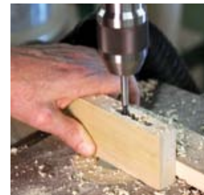
Overlap. The Forstner bit is guided by its edges and won't wander off course when removing the waste between the first set of holes.
