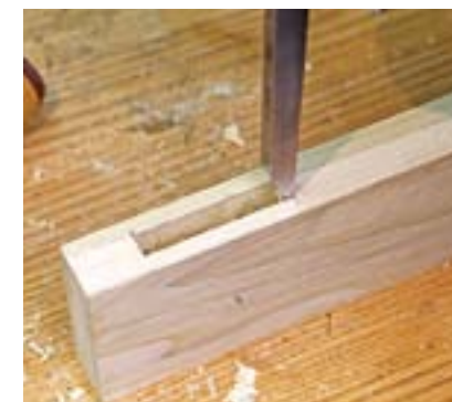
Cleanup time. It takes several cuts to square off the end with a conventional chisel. Position an appropriately sized mortise chisel in a knife line and you can do it with one cut.
