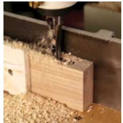
One way out. Chips are pulled up by the bit and exit through the slot in the chisel. Insert the chisel so the slot is facing forward; if it's sideways, the hole will fill up with chips.
