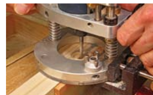
Hole strategy. Make a full-depth plunge at each end of the mortise, locating the cutter to the layout lines. Then make a series of progressively deeper passes in between.
