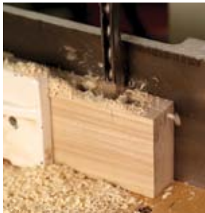
First in. The drill bit does most of the work and leads the way for the chisel to cut the straight surfaces.
