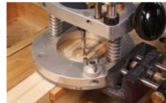
On your mark. Set the tool to the layout line and avoid the need to measure more than one time. Clamp parts together to provide a stable platform for the router.
