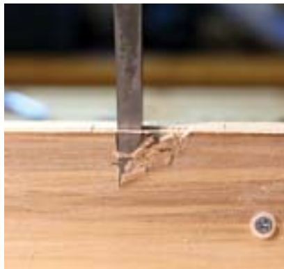
Dig deeper. After the first cut, chips and debris fall into the previous cut, allowing the chisel to go deeper with the same motive force.
