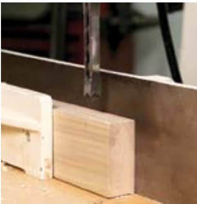
Down low. Clearance between the auger bit and hollow chisel is essential for the tooling to operate efficiently. Don't worry about leaving a ragged bottom.
