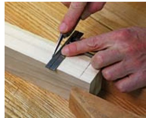
Twofer. Ganging parts for layout ensures that joint locations will be identical, and it saves time. A knife marks a more definite line than a pencil.
