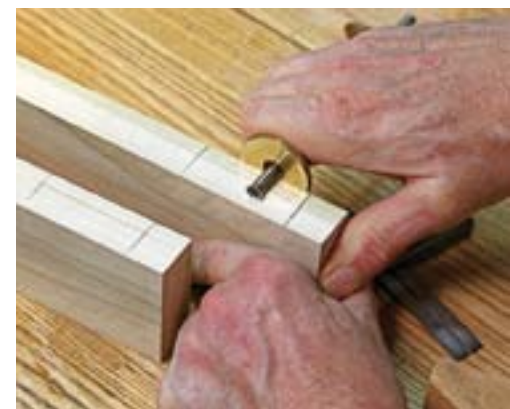
Wheel simple. A marking gauge defines the finished edges of the mortises and is faster and more accurate than repeated measuring.
