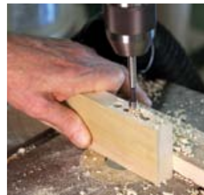
Use a fence. At the drill press the fence provides for consistent placement of the Forstner bit. Drill a series of holes with a space in between.
