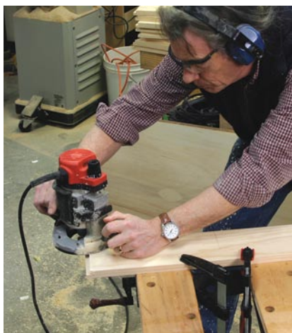
Router rules. Clamp the work securely before routing the rabbets and keep the base firmly on the surface.
