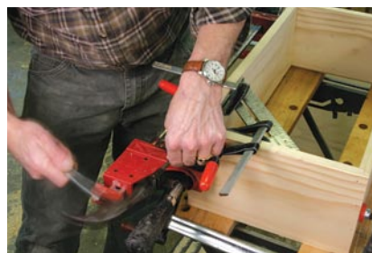
Nice and square. Clamp a square in the corner to hold the boards in position while you drive and set the nails.
