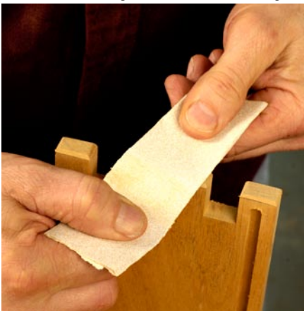
Soft Finish. With a piece of folded #120-grit sandpaper, shape the pillow effect on the end of the fingers removing the previous bevel but not going beyond it. Finish off the short edges with your thumb backing up the sandpaper. Run through the grits refining the pillow shape along the way and ending at #320 grit.
