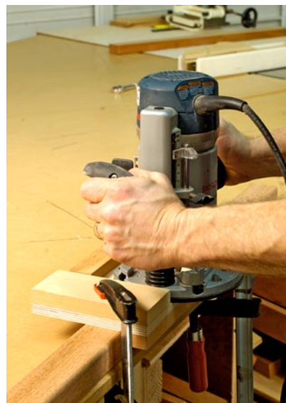
One way only. The router base is trapped by the fences so that it will only move in to the leg.
