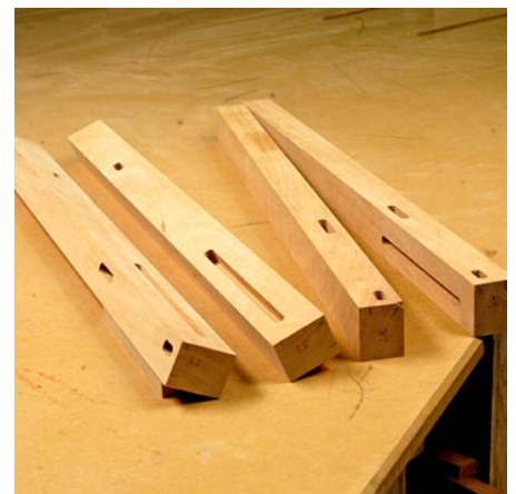
Routing results. Each leg has short mortises for rails and long mortises for panels. Mark the legs on top with their orientation in the table.
