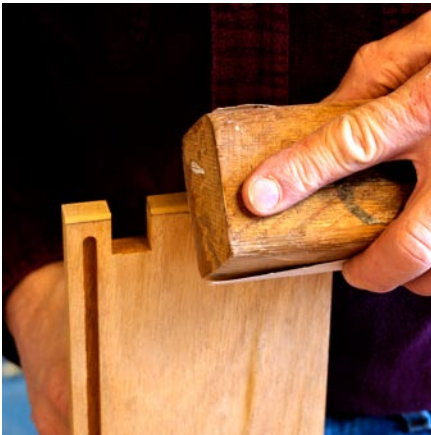
Down to the line. With #120 grit and a sanding block, bevel the edges to the line at a 45° angle.
