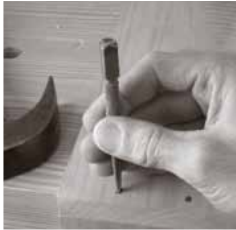
This is the proper way to hold a nail set. Resting your hand on the work helps reduce mis-strikes.
