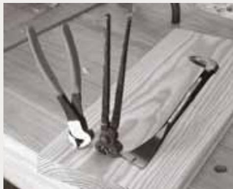
Traditional and contemporary pincers are better at pulling the nails used in furniture-scale work. I wish the handles on the pincers made by Crescent (left) were a bit straighter, but they're far better than most. The Tiger Claw (right) is another useful tool for taking things apart.
