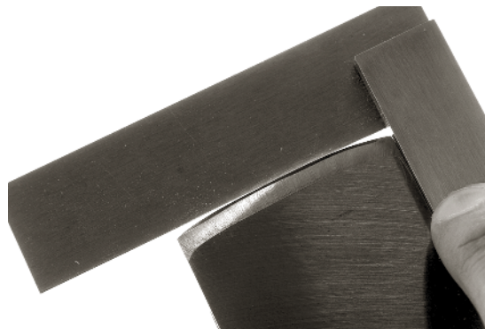
A SILHOUETTE OF THE SHAPE OF my fore plane's cambered iron. It's an 8" radius, which allows me to take an almost 1/16"-thick shaving in softwood.
