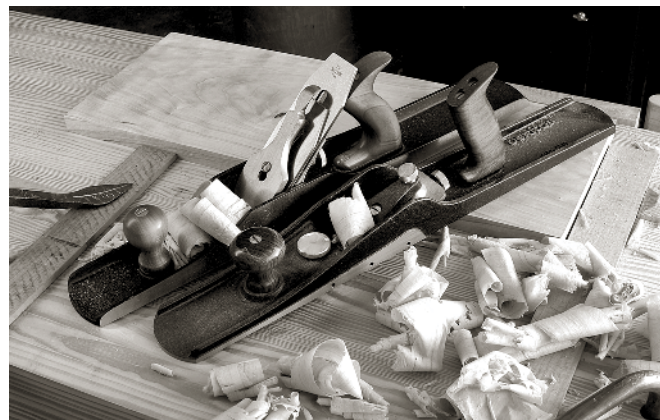
A JOINTER PLANE'S MAJOR ASSET is the length of its sole. The longer the sole, the flatter your board will become. Shown is a Lie-Nielsen No. 7 plane (left) and the Veritas bevel-up jointer. The jointer I covet (not shown) is the Clark & Williams jointer, which can be as long as 30".
