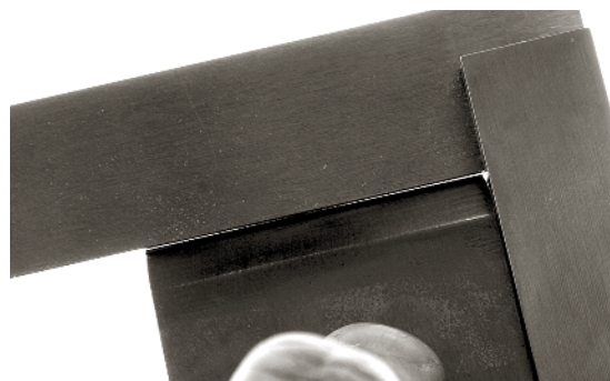
A SILHOUETTE OF A SMOOTHING plane iron. The camber is slight: .002" or maybe a little more.
