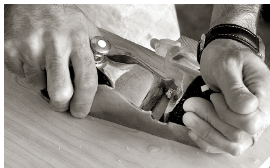
SMOOTHING PLANES REMOVE WISPY SHAVINGS and prepare a surface for finishing.
