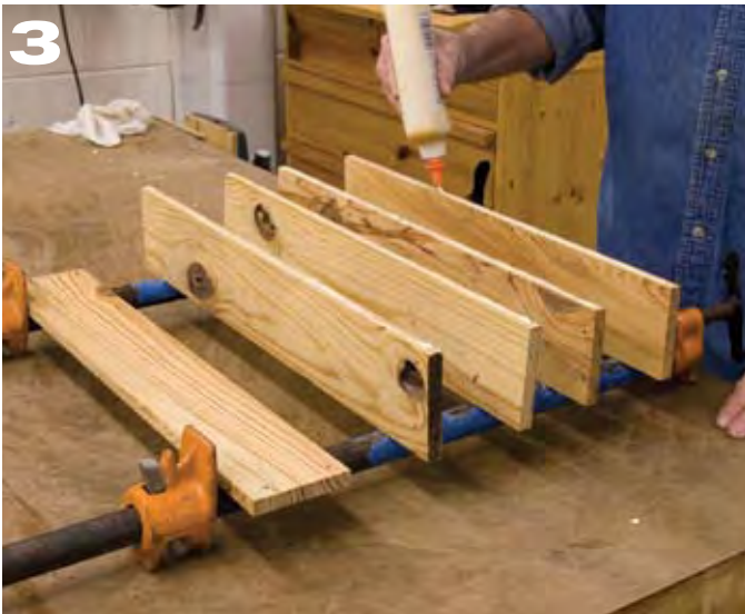
3 Glue up the panels first so the glue can be drying while you work on the leg rails.
