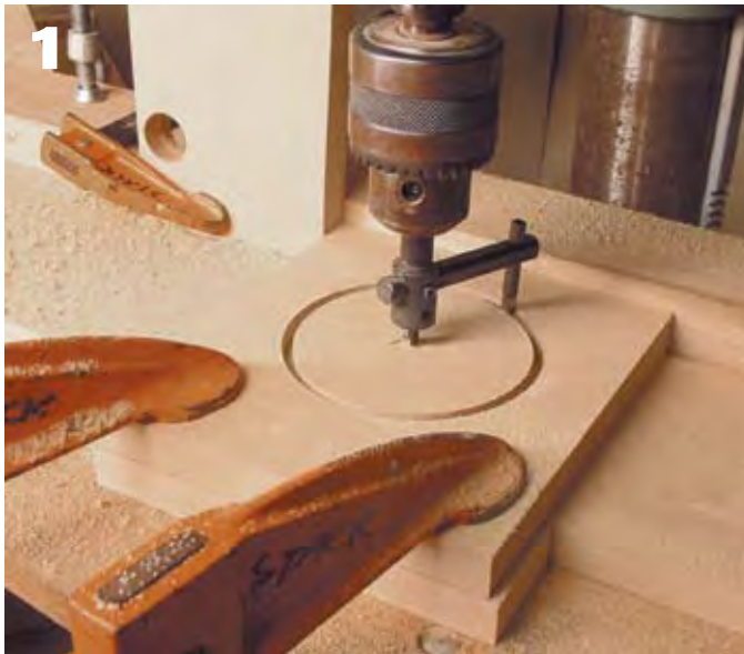
Cut out three collars for the router collar assembly. In each collar, cut a hole larger (add \frac{1}{16} " to the diameter) than the diameter of your router's body.
