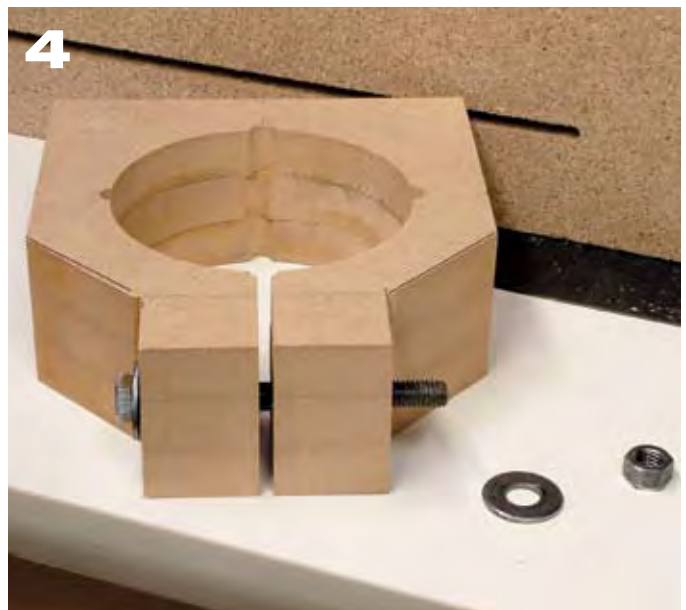
Cut the collar to shape using your table saw or band saw. Then stand the collar on edge and drill a \frac{3}{8} "-diameter hole for the bolt.
