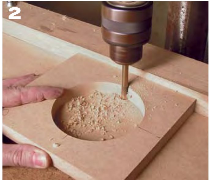
If your router has those little tabs on its body like mine does, you'll need to cut out for those so the collar will slip on the router's body smoothly.
