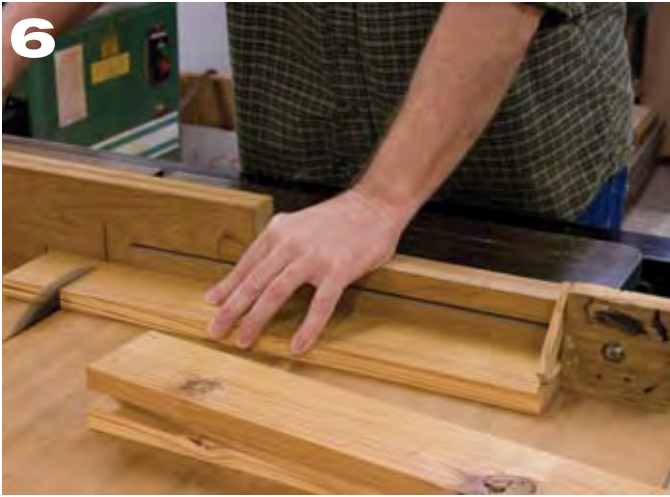
6 Cut the rails to length. Be sure to allow for the 1" tenons. Notice the flipper on my stop. I flip it up and slide the part under the flipper. This makes the cut about 1/4" longer than the final length.
