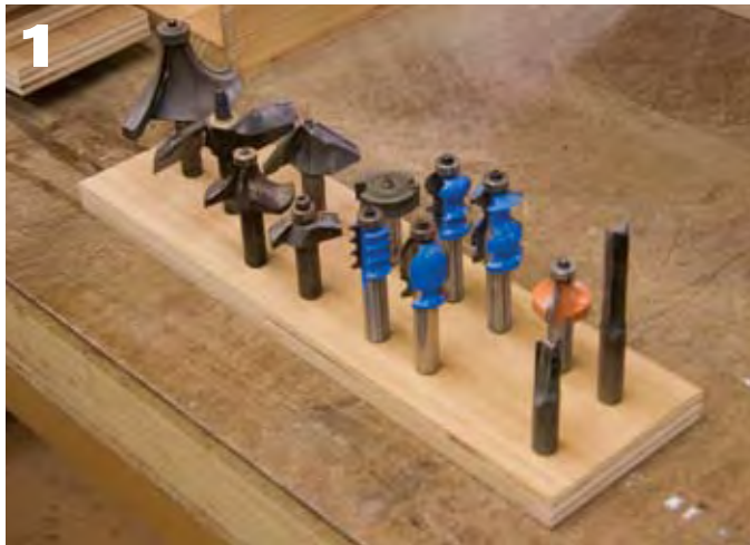
1 Cut out the pullout parts. Arrange your bits on the shelves. These are the largest cutter I have and they all fit on one shelf. I marked the hole locations and drilled them about halfway through the shelf.
