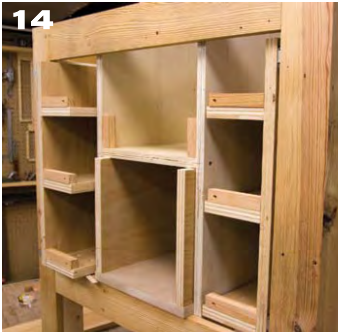
Glue cleats to the pullout shelves, to the sides of the top space and to the sides of the drawer (I haven't glued these in place yet).
