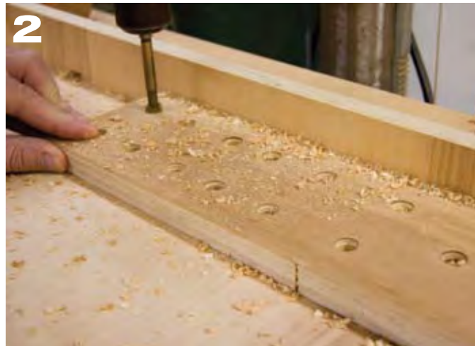
2 I drilled the rest of the shelves with two rows of holes spaced fairly evenly, just using my eye to gauge the distance between holes. I drilled three shelves with \frac{1}{2} " holes and the other three with \frac{1}{4} " holes. I ended up with ninety holes total – more than enough for now and the future.
