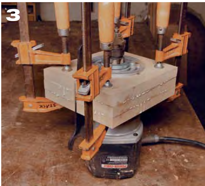
To hold the three collar pieces in alignment, I used my router as a form. Use enough glue to hold the parts together but keep the glue away from the inner edges of the circle cutout if you can. If a little glue does stick to your router's body, simply pop off the dried glue with a chisel.
