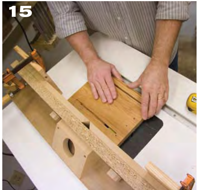
Cut out the drawer front, pullout fronts and the vent panel. Fit them to the front of the router table, leaving about \frac{3}{32} " space between all these parts. Then cut the vents in the vent panel. Here, I am using my old router table to plunge-cut the vent slots.
