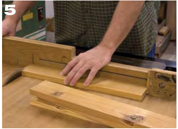
5 When I rotate the part end-for-end, the flipper will drop down. I then butt the part against it and make the final-length cut.
