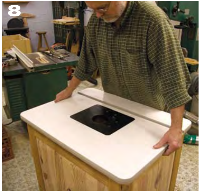
8 Slide the assembled router carriage into the top of the inner cabinet. Hold the tabletop in place and center the hole in the tabletop insert with the hole in the carriage. Mark the underside of the top to locate it on the router table.
