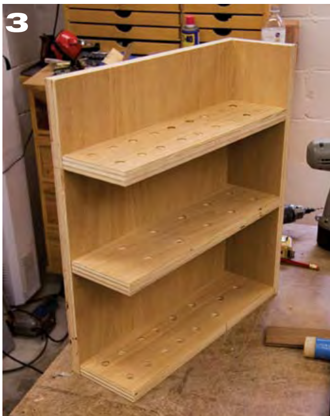
3 Screw the pullout parts together. I made the right-handed pullout for my router bits with \frac{1}{4} " shanks the left-handed pullout for my \frac{1}{2} " bits.
