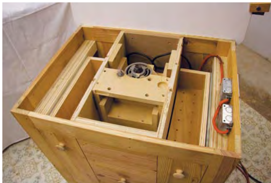
I've removed the two inner tops so you can see what the inside should look when the table is completed. The electric is easily routed along the top pullout spacer and behind the pullout. The inner tops will keep dust out of the pullout cavities.
