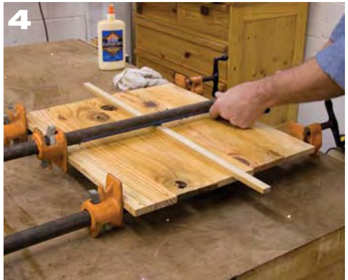
4 Align the pieces and clamp them together. Be sure to have clamps on opposite sides of the panel for even clamping pressure.
