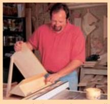
pieces, so check your work. Later you'll add a corner brace that will keep this angle fixed at 90 degrees. Attach the two triangular braces to the side and runners. Attach the braces with nails and glue.
