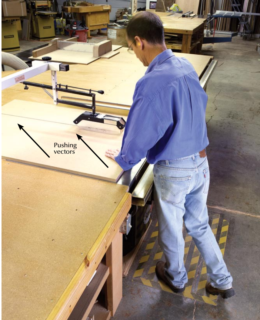
Good posture. Good table saw technique begins with your stance. Always stand to the left of the blade and gain additional support by bracing yourself against the saw.
