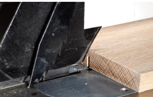
Less-than-stellar design. Due to typical American-style splitters extending above the top of the blade, making any cut except for a cut completely through your stock is not possible.
