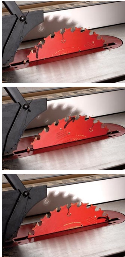
Up, forward and down again. If you follow the marked tooth in the series of photos above, you can see how initially the tooth lifts the work up. Then it pushes it forward. And finally it pushes it down.
