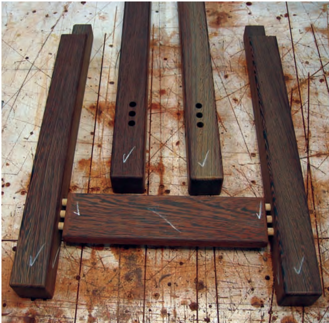
11 Using dowels and waterproof glue, assemble and clamp the leg-and-cross-brace assemblies.
