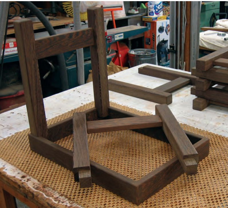
13 The leg assemblies are now ready to be attached to the apron corners.
