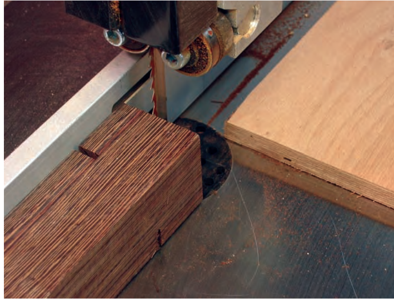
6 Finish the shoulder cuts on the band saw using a stop clamped to the table to limit the length of cut.
